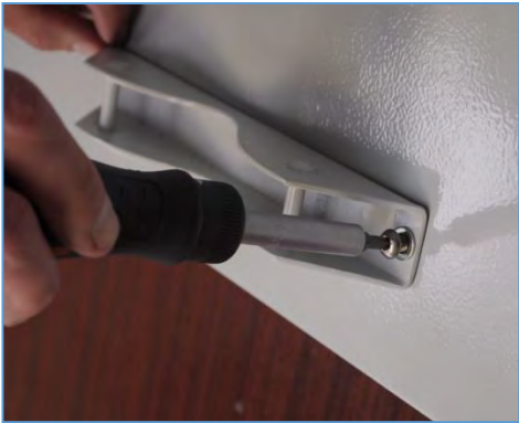
Figures 3 & 4, standard banding bracket mounted directly to sign with M6 tamper-proof screws
